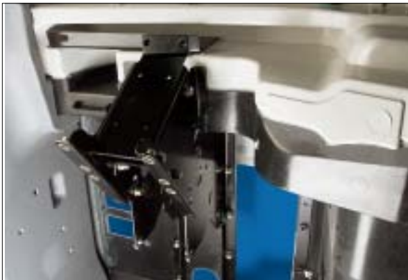
Our firewall assembly illustrates the effective use of lightweight composite and aluminum components combining with bonded and huckbolted construction to form a uniquely strong structural system.
