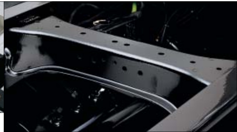
Extensive use of cast aluminum on components such as heavy duty crossmembers has reduced weight without compromising durability.
